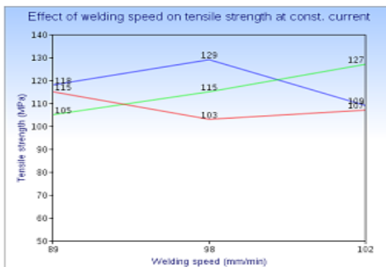
Fig 3: Effect of Welding Speed on Tensile Strength
